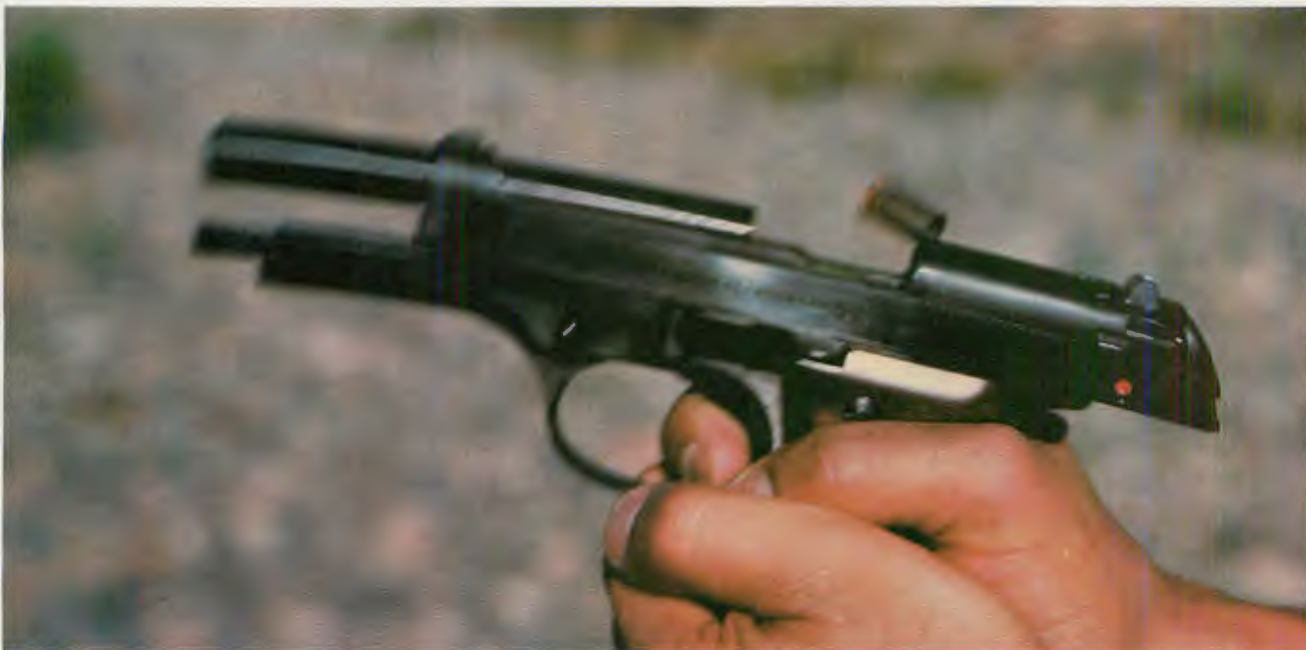
ABOVE: Full-open top of 92 SB slide eliminates malfunction from ejection port restriction. LEFT: Ambidextrous safety allows strong-or weak-hand use, right side view shows exposed ejector. RIGHT: Falling block lock assembly shows debt to Walther P-38. LOWER LEFT: Lever to
